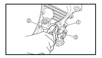
• Install the bearing ① onto the yoke.
