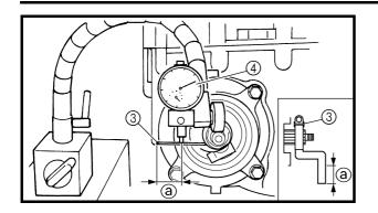
• Attach the gear lash measurement tool ③ and dial gauge ④.
