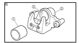
Brake fluid delivery passage (brake caliper body)
