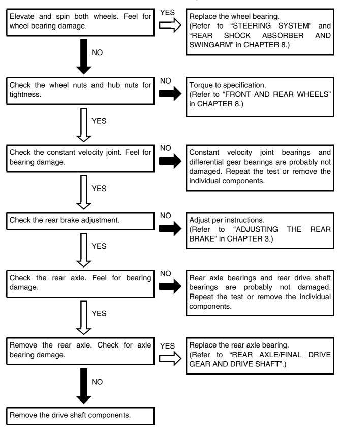
FRONT CONSTANT VELOCITY JOINTS AND DIFFERENTIAL GEAR
