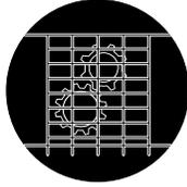
Never remove the covers guarding personnel from rotating parts, when the engine is operating.
