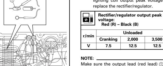
Make sure the output lead (red lead) ① of the rectifier/regulator is disconnected when measuring the output peak voltage.
