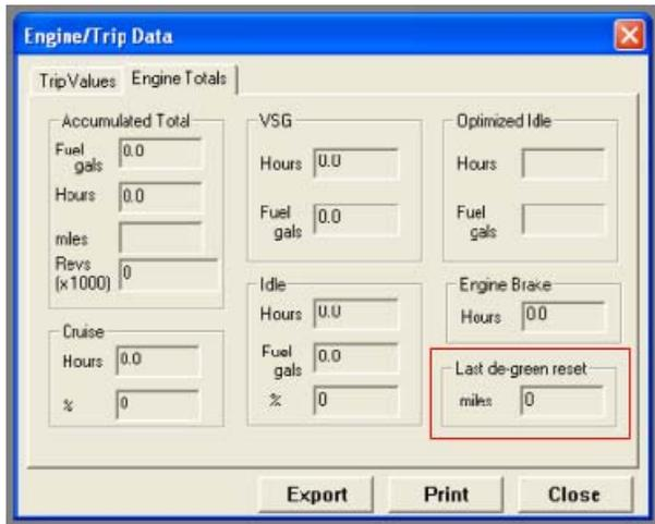
4. The user may review how many miles the engine has run since the last de-green process was completed by choosing the “Engine / Trip Data” option form the “Tools” drop-down menu. The information is contained on the “Engine Totals” tab in the lower right corner.
