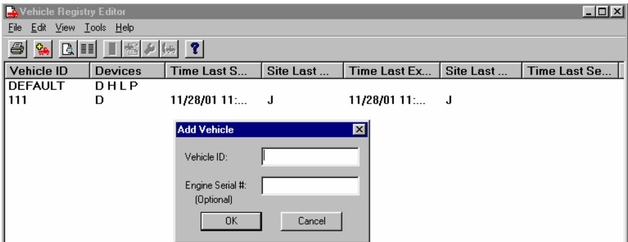
Enter the ID. (If you want to check for an existing Vehicle ID, you can retrieve the calibration in DDDL and check the “Vehicle Unit Number” on tab 1 prior to beginning this process.) Click on “OK”.
