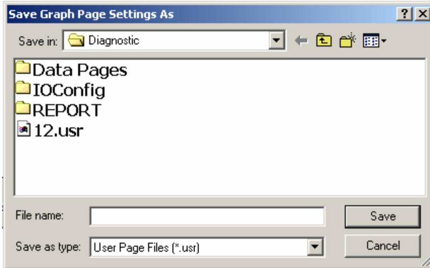
If you wish to save this selection for future use select the “Save” box on the main Graph window and select a file name in the dialog box that appears. The selection may be recalled at a later time by choosing the “Load” box on the main Graph window.
