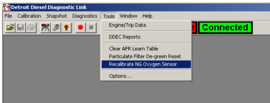
I. Go to the “Tools” drop-down menu and choose the “Recalibrate NG Oxygen Sensor” item. This item will only be available for use with DDEC natural gas engine and will appeared “grayed out” in other DDEC application,
