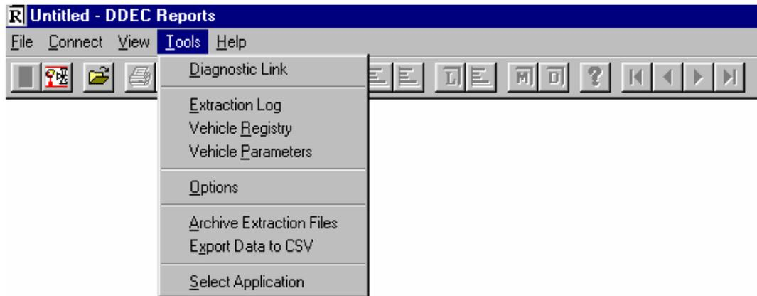
3. The Vehicle Registry Editor will appear on your screen. If you have already extracted data from this vehicle before, double click with you left mouse button on the vehicle you wish to modify in the “vehicle ID” column and you’ll be taken to the “Vehicle Details” screen (move directly to step 5). If you have never extracted data from the vehicle before, you’ll need to set up the vehicle in the vehicle registry. Click on the truck / plus sign icon and you’ll be prompted to enter the vehicle ID.
