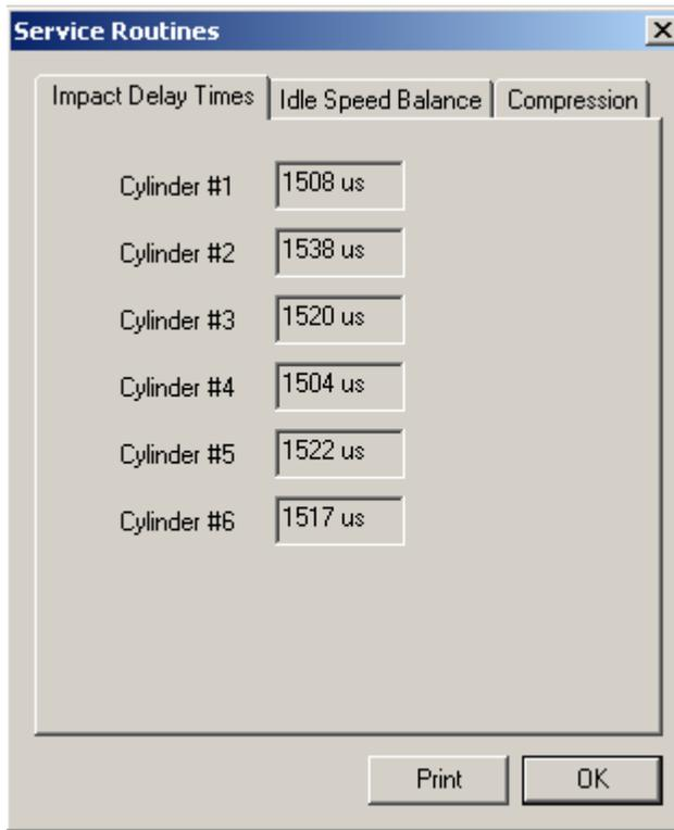
The screenshot shows a dialog box titled "Service Routines" with three tabs: "Impact Delay Times", "Idle Speed Balance", and "Compression". The "Impact Delay Times" tab is selected, displaying a list of six cylinders with their respective impact delay times in microseconds (us). The values are: Cylinder #1 (1508 us), Cylinder #2 (1538 us), Cylinder #3 (1520 us), Cylinder #4 (1504 us), Cylinder #5 (1522 us), and Cylinder #6 (1517 us). At the bottom of the dialog are "Print" and "OK" buttons.
