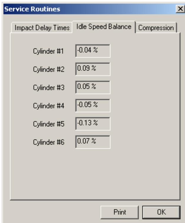
The screenshot shows the same "Service Routines" dialog box, but with the "Idle Speed Balance" tab selected. It displays the deviation values for each of the six cylinders in percent (%). The values are: Cylinder #1 (-0.04 %), Cylinder #2 (0.09 %), Cylinder #3 (0.05 %), Cylinder #4 (-0.05 %), Cylinder #5 (-0.13 %), and Cylinder #6 (0.07 %). "Print" and "OK" buttons are visible at the bottom.
