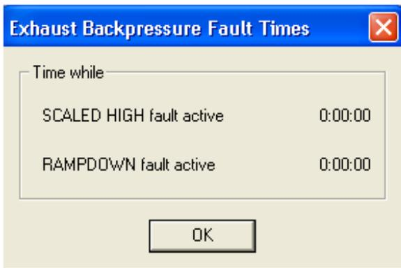
Beginning with version 4.20 you may view the exhaust backpressure fault times on DDC Series 2000 and 4000 series engines that support this feature. Choose Exhaust Backpressure Fault Times from the Diagnostics menu.
