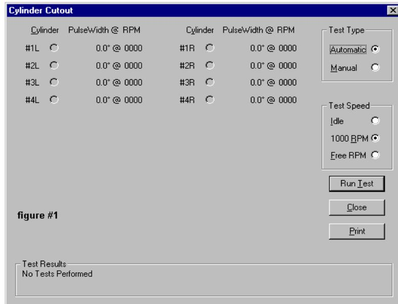
1. From the Diagnostics drop-down menu select the “Cylinder Cutout” option. The cylinder cutout screen in the figure above will appear on your screen.
