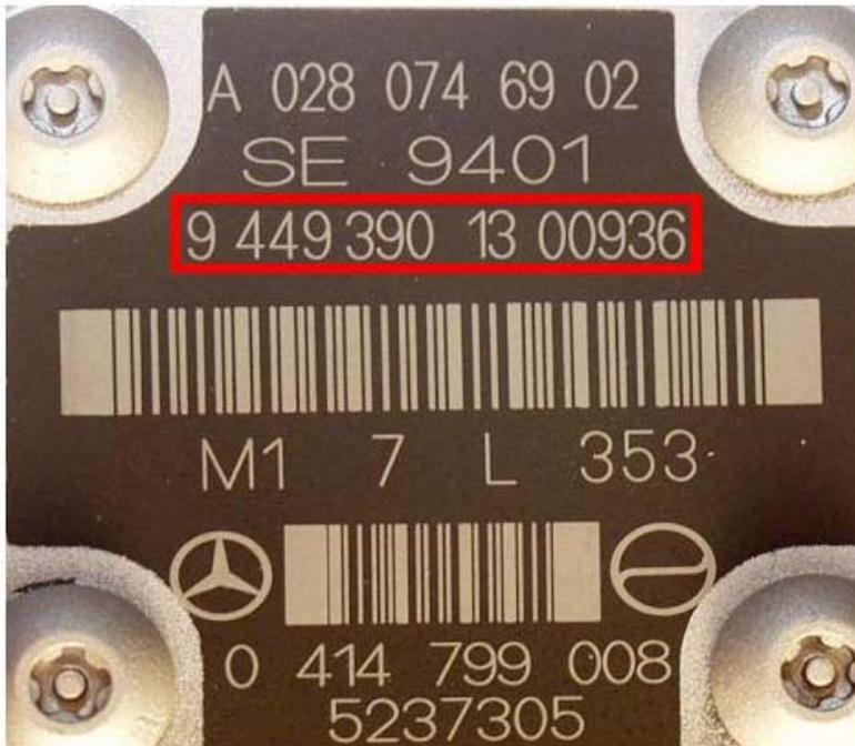
1. The number has always been on this particular part however with the release of the 2004 MBE engines there is a requirement to enter this information when the unit is replaced. You may use do this with the Programming Station, Detroit Diesel Diagnostic Link, or the Minidiag. The routine to perform this operation in the Minidiag is called “Routine 006 - pump line nozzle change”. To enter the value with DDDL choose the “Calibration” drop-down menu and select “Injector”.
