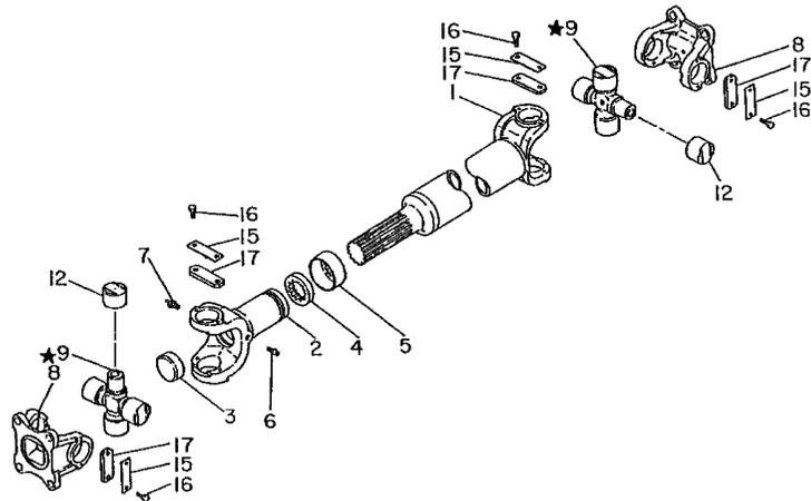
KEY NO. 1 - 17 SHAFT ASSY - PROPELLER (ASSY KEY NO.100)
